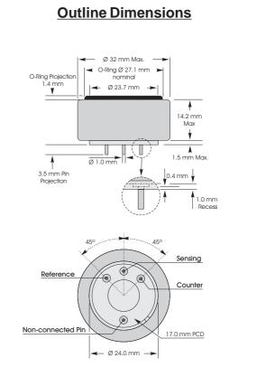
All tolerances ±0.15mm unless otherwise stated. Do not solder to pin connections
